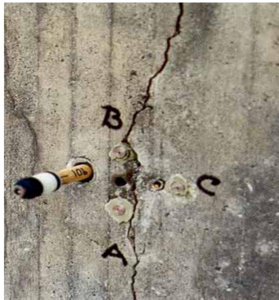
Fig. 9: Location with expansion and humidity measurements, Elgeseter bridge.
